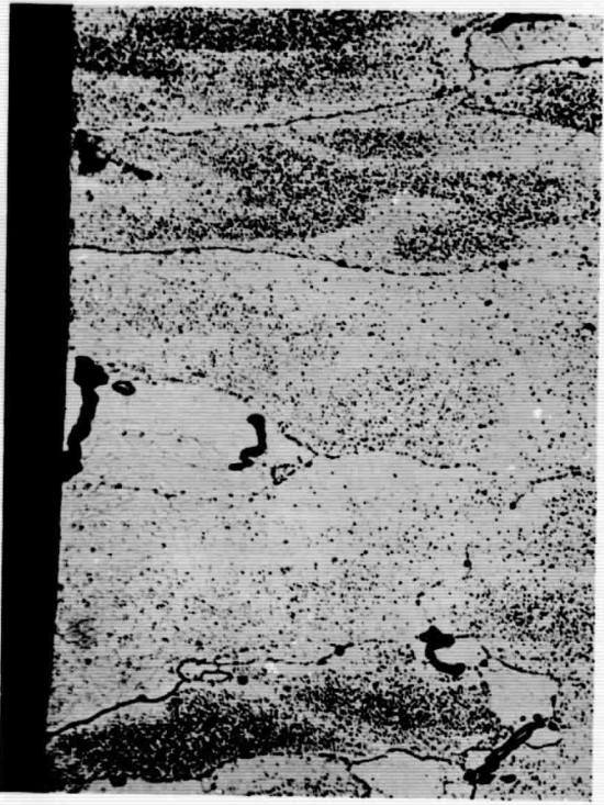
Development of pitting attack in 7039-T6 plate exposed unstressed to pH2 solution of 0.5N NaCl + 0.5N Na 2 CrO 4 (X500).
