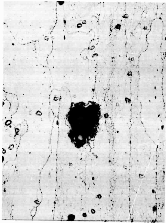
Pitting of 7075-T73 stressed short transversely to 75% YS and exposed to 1N KHF 2 at pH2 (X500).
