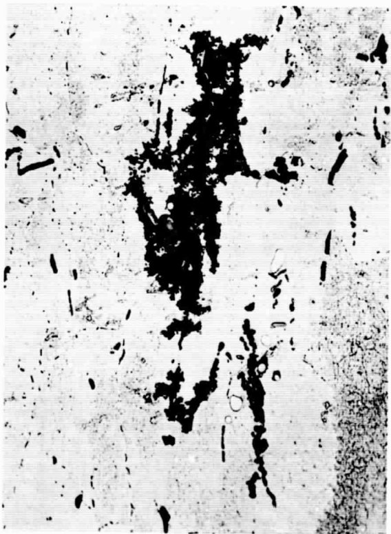
Pitting of 2219-T87 stressed short transversely to 75% YS and exposed to 1N NaCl adjusted to pH2 with H 2 SO 4 (X500).
