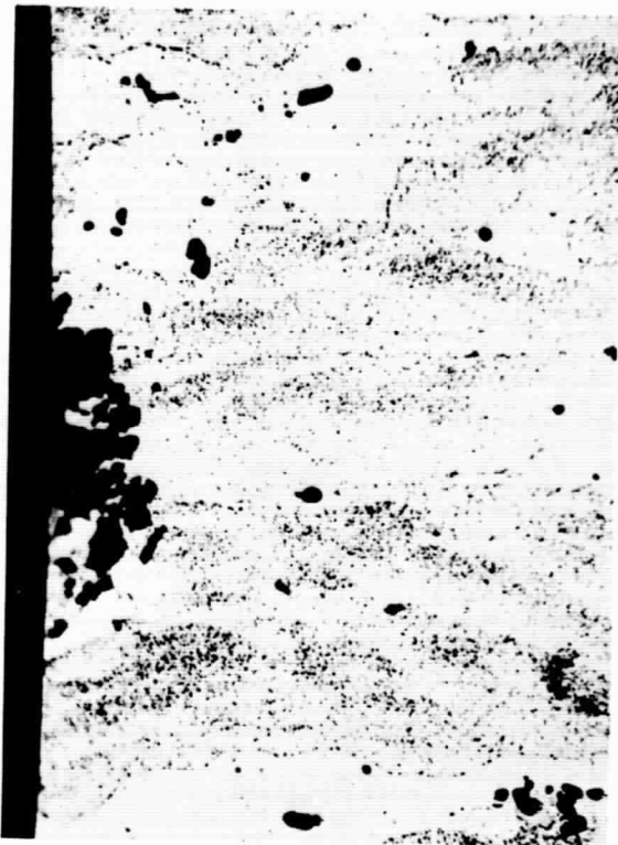
Tuning fork specimen of 7075-T73 stressed short transversely to 75% YS and exposed to 1N NaCl solution adjusted to pH2 with HCl. (X500)
