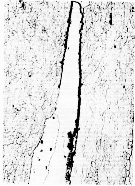
Crack initiation and development in 7075-T6 stressed short transversely to 75% YS and exposed to 0.5 NaCl + 0.5 Na 2 SO 4 solution at pH2. (X500)
