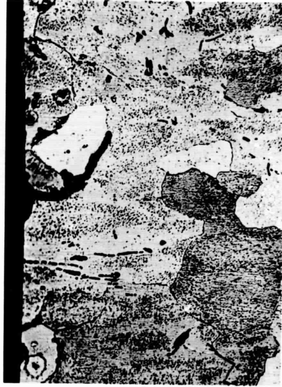
Selective attack in 2219-T37 stressed to 75% YS S.T. and exposed to 1N Na 2 SO 4 solution at pH2 (x500).
