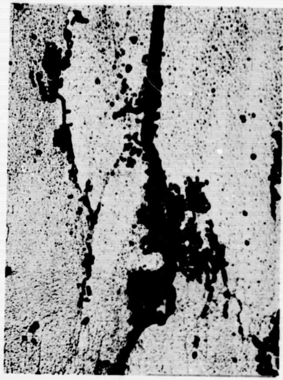
Crack initiation in 7079-T6 plate stressed short transversely to 90% YS and exposed to pH1 NaCl- AlCl_3 solution (X500).
