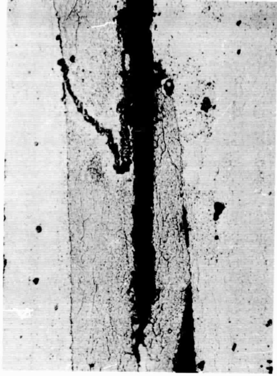
Crack development in 7075-T6 stressed short transversely to 75% YS and exposed in 4N NaCl + 0.5N KNO 3 solution at pH 0.4. (X500)
