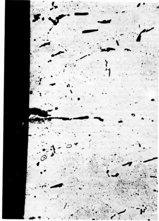
Attack of 2219-T87 stressed short transversely to 75% YS and exposed to 1N KHF 2 at pH2 (X500).
