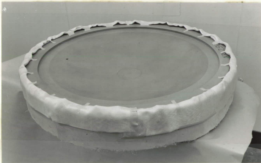
Figure 10. Assembly of Fiberglass Hatch Dome
