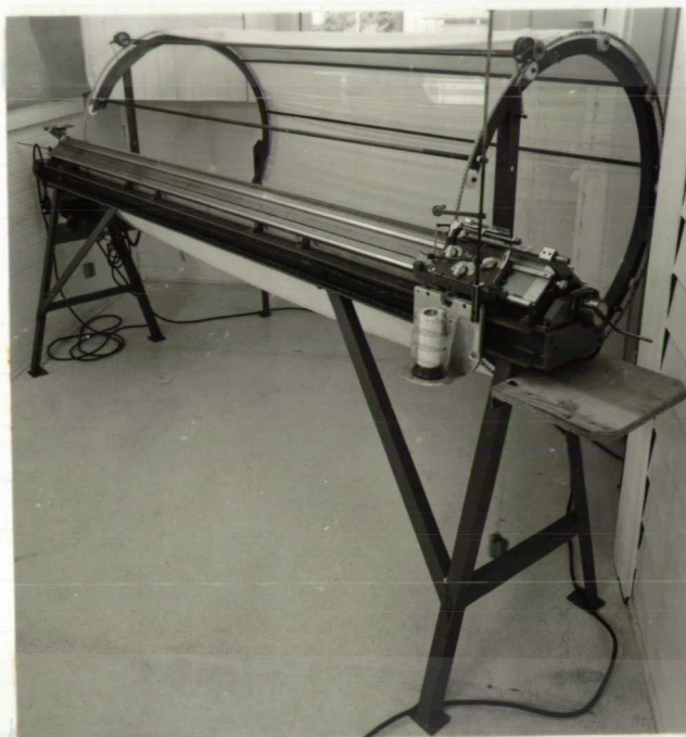
Figure 13. Astroflex Knitting Machine with End Rings Installed
