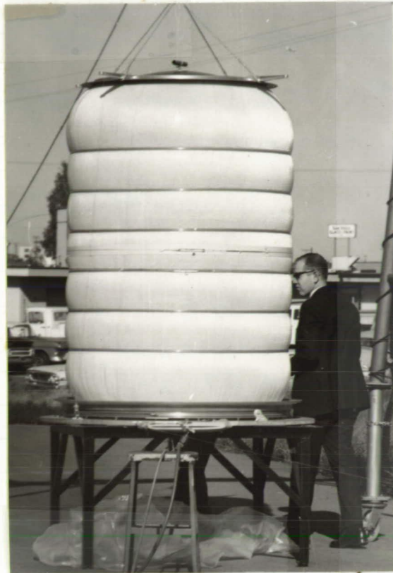
Figure 25. First Proof Pressure Test Sequence
