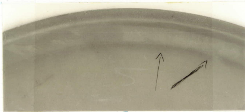
Figure 29. Delaminations in Hatch Rings
