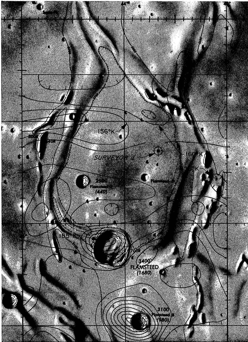
Fig. IV-1. Isotherms in landing site region during totality of lunar eclipse (Ref. IV-1)
