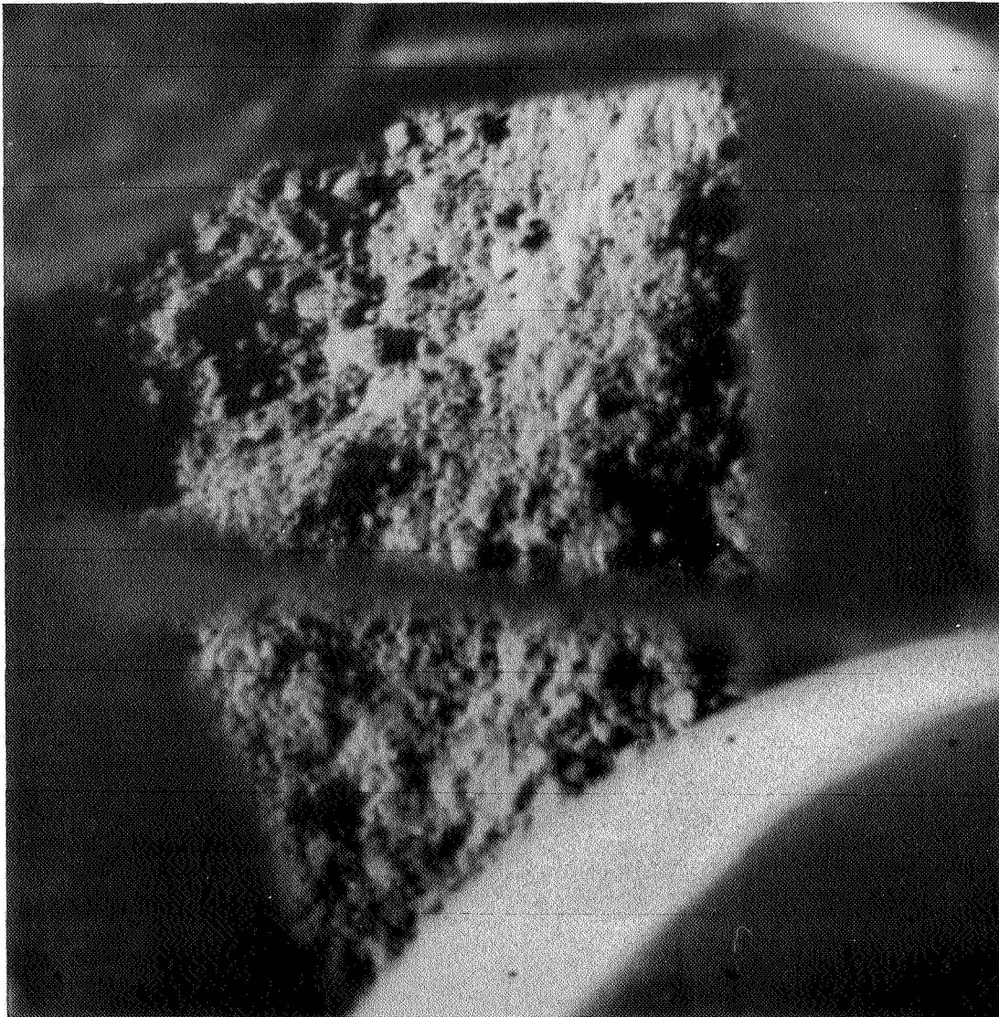
Fig. VI-13. Block assembly imprint taken late on the second lunar day. (Sun angle is 22^\circ and from the left of picture. No noticeable change in the disturbed material has been observed during a time period greater than 5 wk.)
