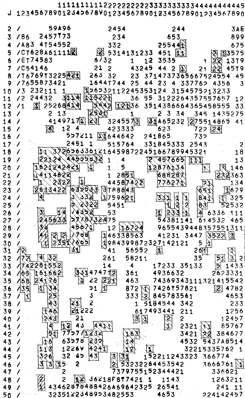
Figure 6. Portion of Interfacial Flow Map. Rows and columns are Indicated and the sequence of gap height increments is 1, 2, ---, 9, T, A, B, ---. Contact is indicated by a blank.
