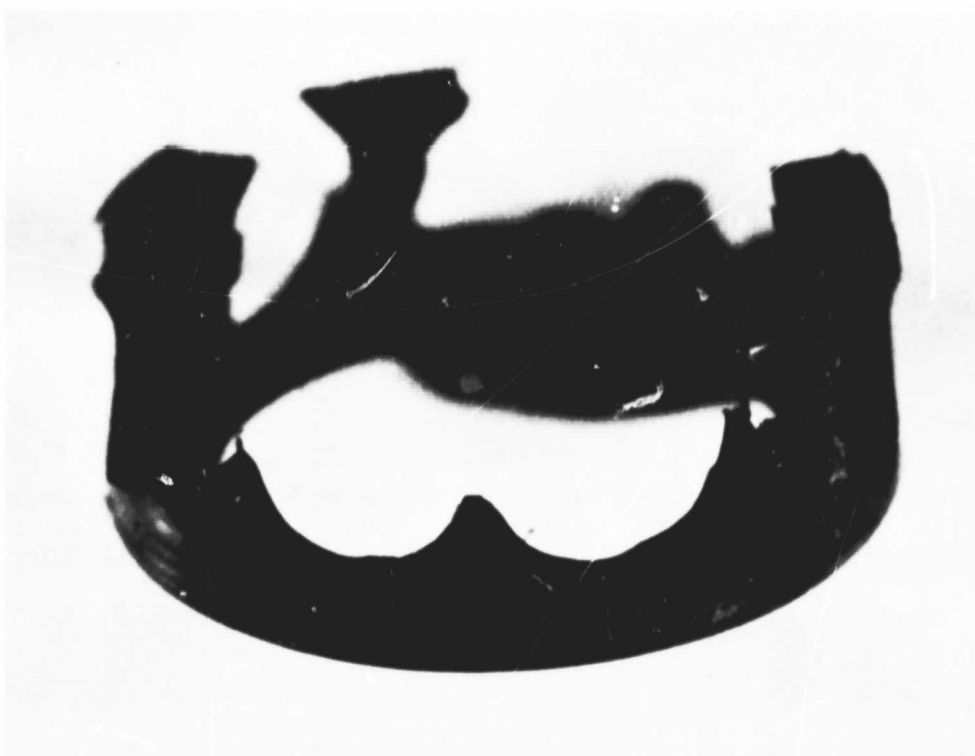
COMPLETE WEAROUT OF ONE SIDE OF RETAINER
