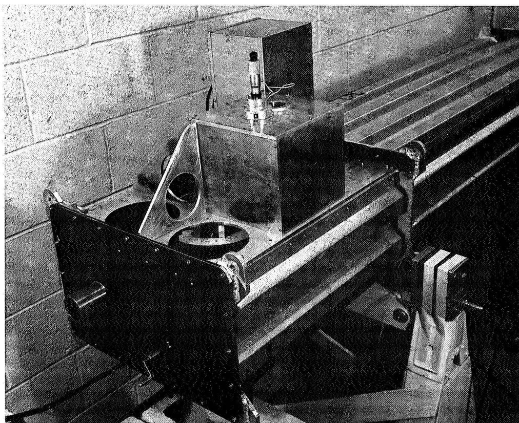
Fig. 2 Focal plane end of 4-meter spectrometer containing entrance slit (with chopper in front), grating and drive, and detector mounted in cold box. Micrometer screw seen on top for focusing detector; small crank at bottom, for hand setting of grating position.
