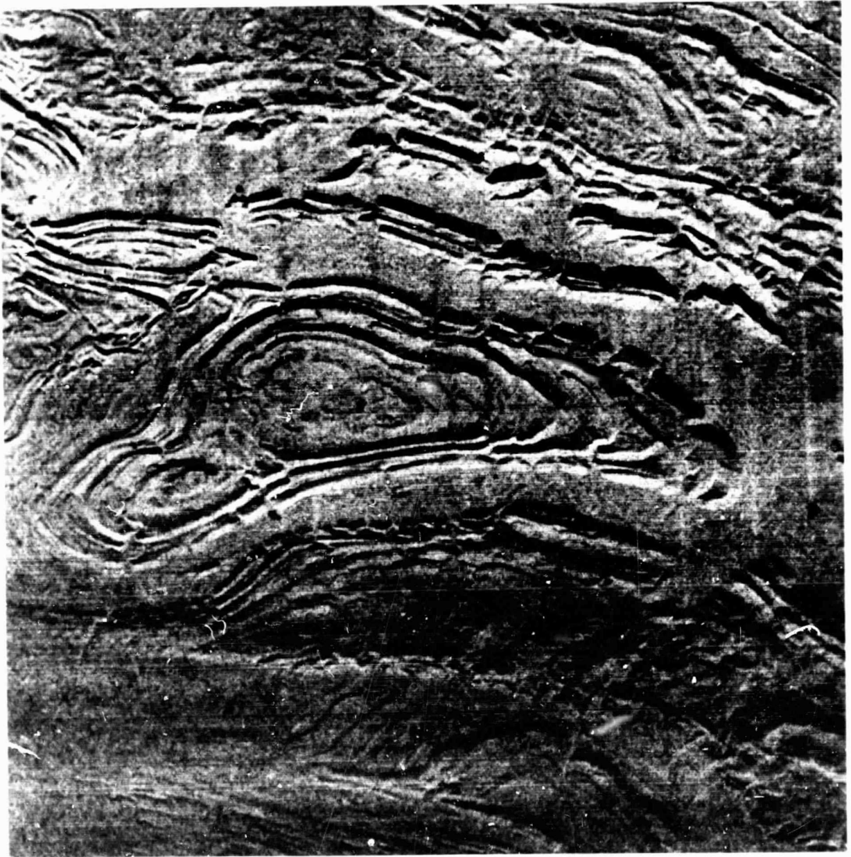
FIGURE 5. This radar image of the Tuskahoma syncline, Ouachita Mountains, Oklahoma, clearly shows the gross landform pattern better than it appears on conventional photography.
