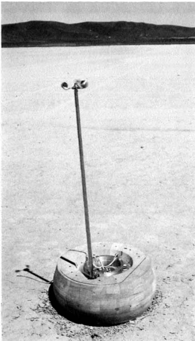
Fig. 4. Anemometer and CSAD capsule after drop test
