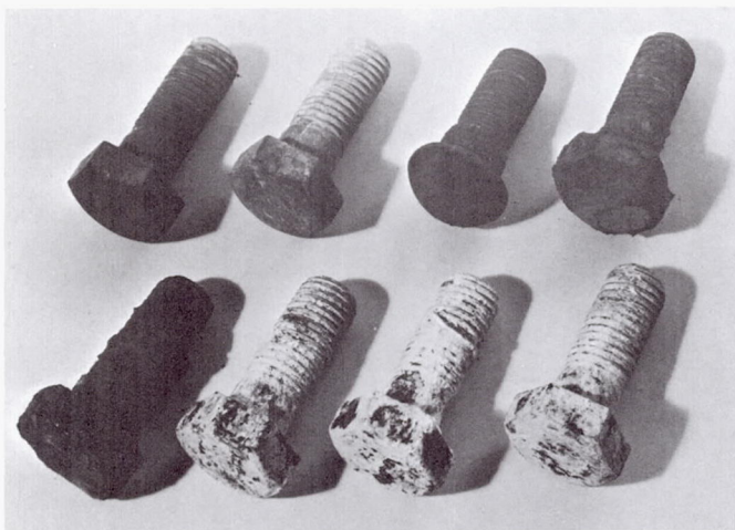
Fig. 7. Typical bolt specimens after 1000-h salt spray exposure
