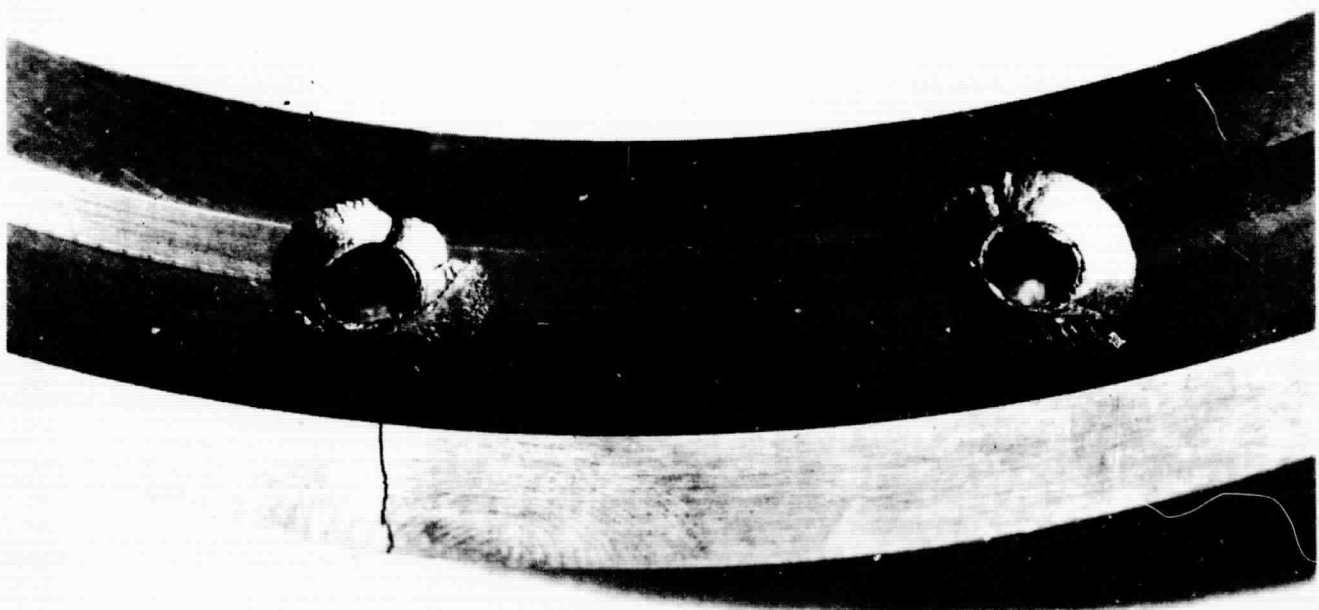
Fig. 37 - Beryllium Ring (Upper) and Close-Up View of Cracked Portion (Lower).
