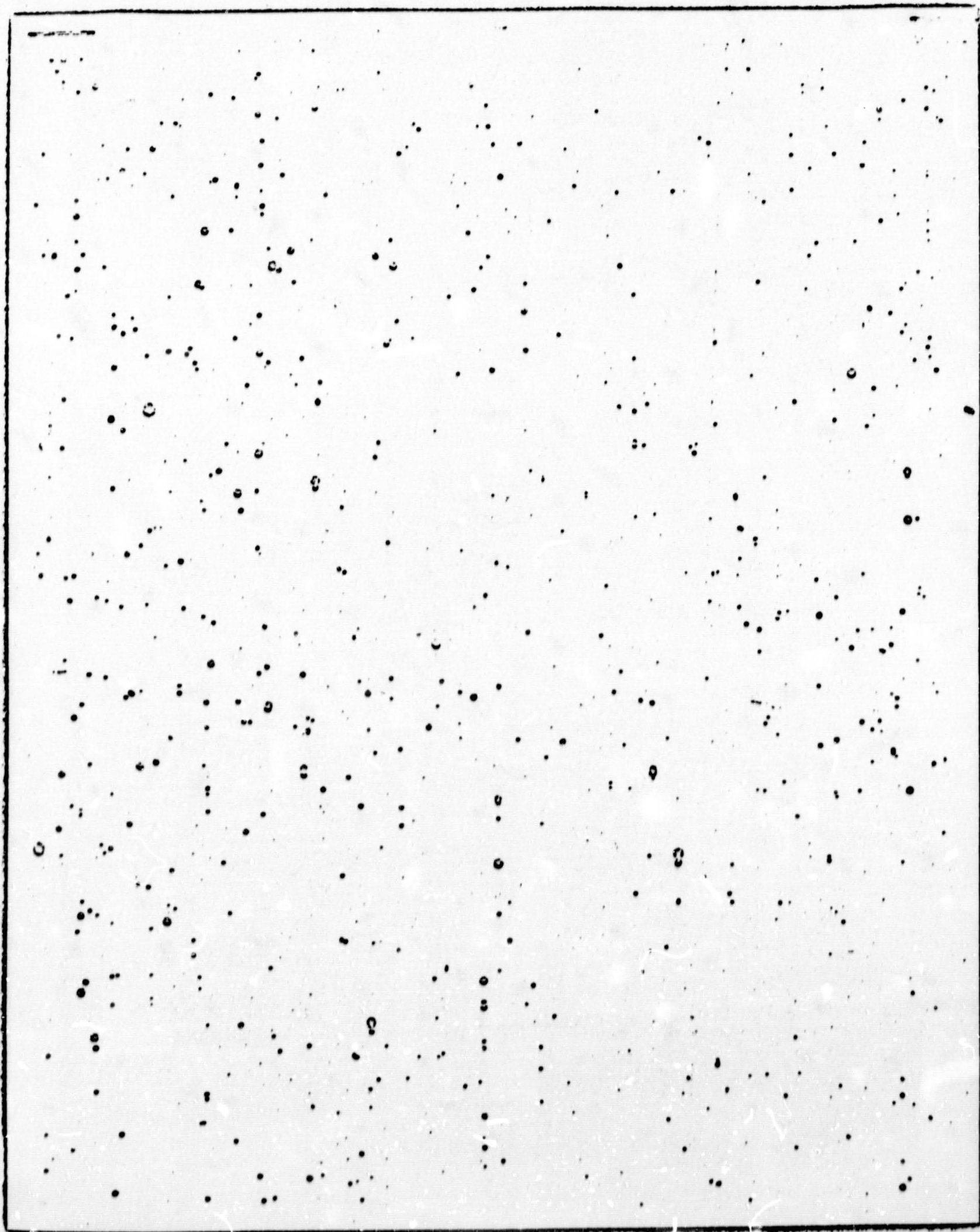
Exhibit 2 Pinhole Frequency Photograph Republic Foil Corporation .00025 Electrodry Aluminum Foil Photo #2 Case #16895 Roll #2
