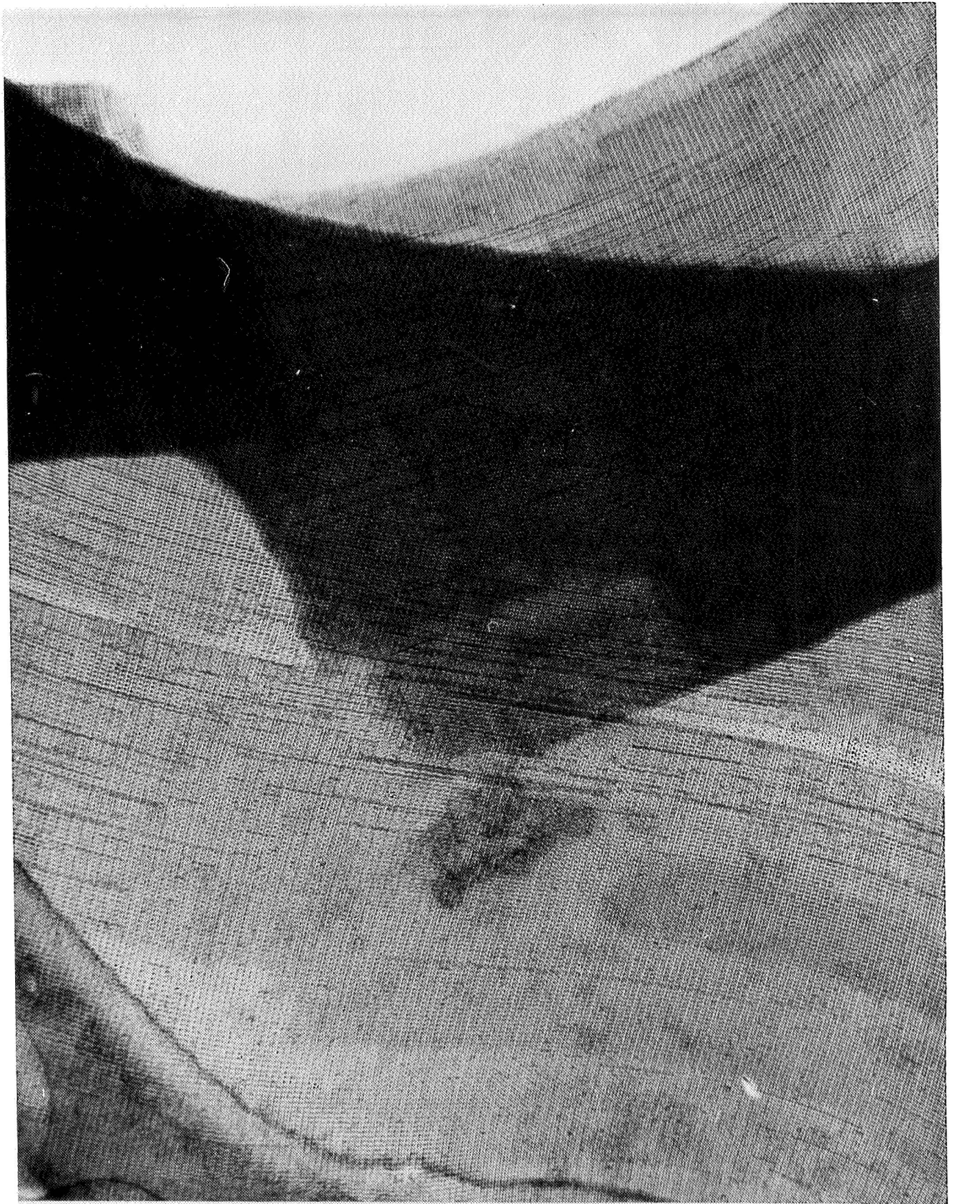
HIGH RESOLUTION ELECTRON MICROGRAPH OF THICK (ca. 400Å-500Å) CATALASE PROTEIN CRYSTALS STAINED WITH URANYL FORMATE, SHOWING LATTICE SPACINGS IN VARIOUS ORIENTATIONS WITH REDUCED RADIATION DAMAGE, RECORDED WITH 200 KV HU-200E HIGH VOLTAGE ELECTRON MICROSCOPE PROVIDED WITH HIGHLY STABILIZED CENTRAL POWER SUPPLY. (Electron Microscopy by M. Ohtsuki, Photography by Charles Hough, Laboratory of Dr. H. Fernandez-Moran, University of Chicago)
