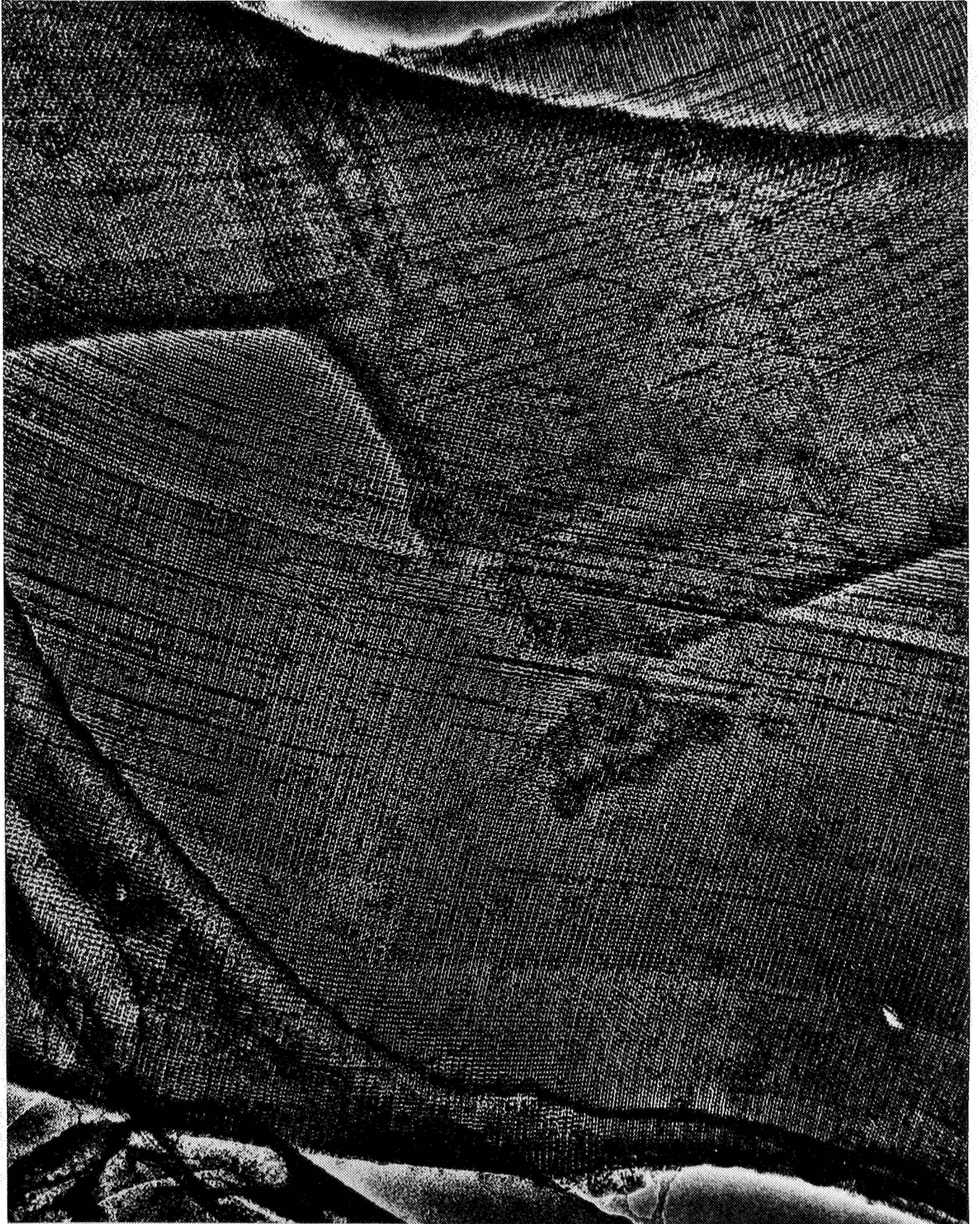
HIGH RESOLUTION ELECTRON MICROGRAPH OF THICK (ca. 400Å-500Å) CATALASE PROTEIN CRYSTALS STAINED WITH URANYL FORMATE, SHOWING LATTICE SPACINGS IN VARIOUS ORIENTATIONS WITH REDUCED RADIATION DAMAGE, RECORDED WITH 200 KV HU-200E HIGH VOLTAGE ELECTRON MICROSCOPE PROVIDED WITH HIGHLY STABILIZED CENTRAL POWER SUPPLY. (Electron Microscopy by M. Ohtsuki, Photography by Charles Hough, Laboratory of Dr. H. Fernandez-Moran, University of Chicago)
