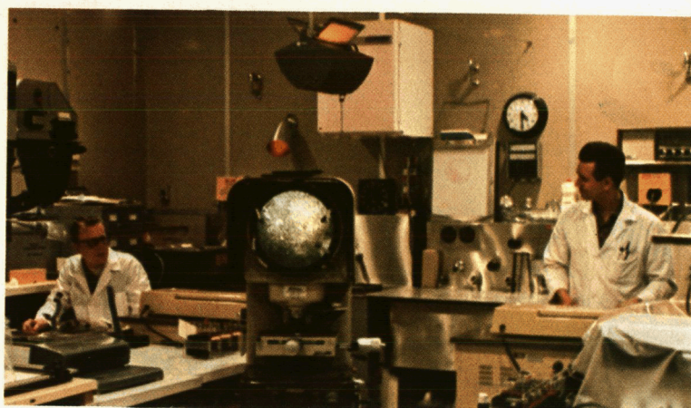
Thin layer of metal is deposited on specimens in ultrahigh vacuum, left . Photographic laboratory, above , includes shadowgraph on which projected image from the microscope can be studied in detail.
