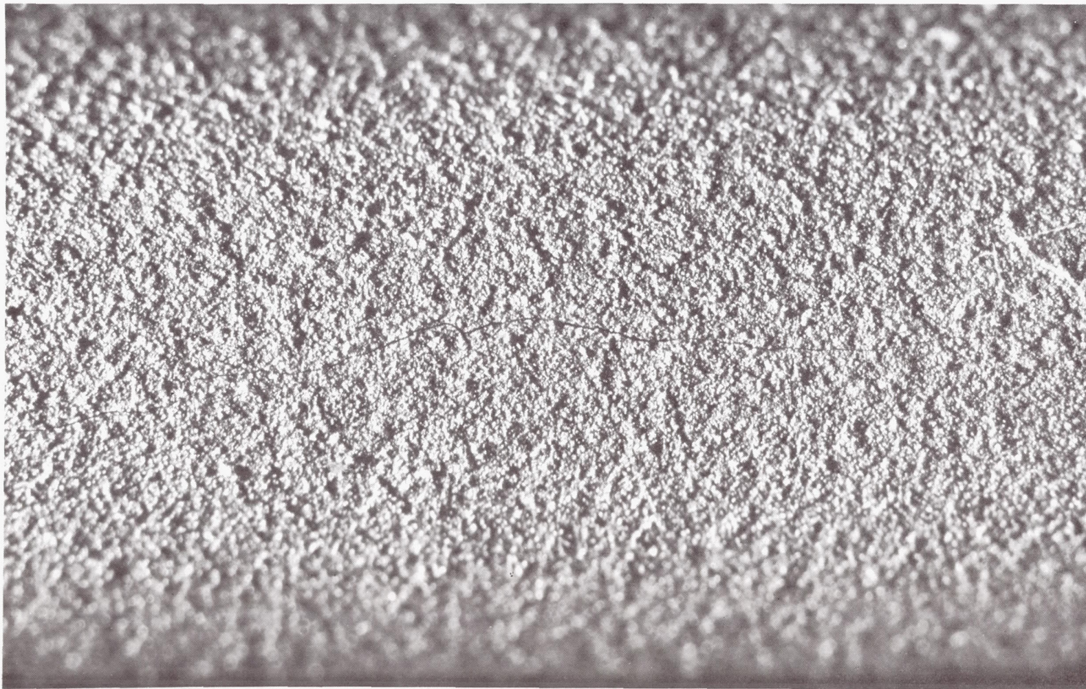
Figure 78 Close-up View of Surface of Iron-Titanate-Coated Columbium-1 Percent Zirconium Tube After Thermal Cycling in Vacuum Between 1500°F and 1900°F for 10,000 Hours Showing Crack in Coating Outside of Test Section
