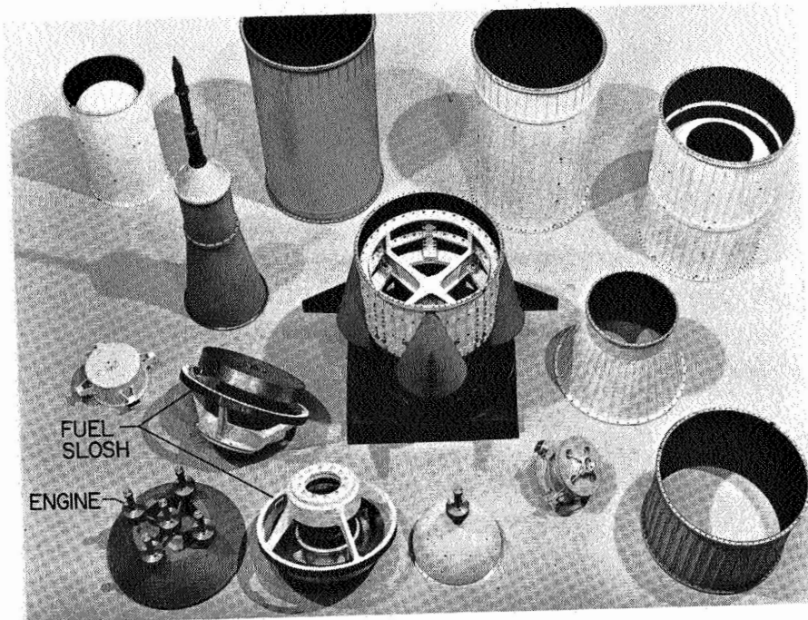
Figure 19.- 1/40-scale model details of Saturn V.
