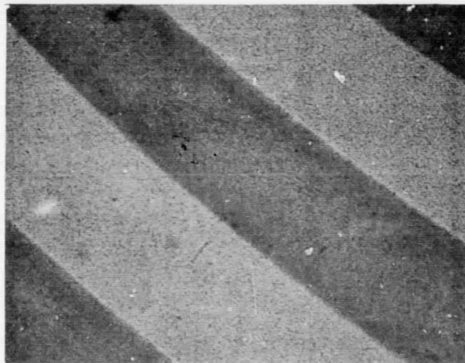
Fig. 17b Whipple grooves machined in vapor plated alumina by ultrasonic machine technique (100 X).
