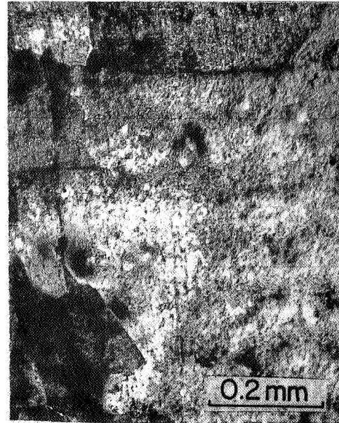
(d) After Reversed Creep, T=0.70T_m , \tau_a = \pm 280 psi, \Delta\gamma=0.030
