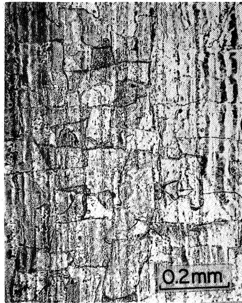
(b) After Reversed Creep, T=0.5T_m , \tau_a = \pm 640 psi, \Delta\gamma=0.047
