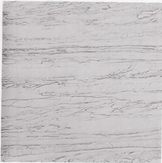
(c) Swaged W-1.5Hf capsule. Murakami's etchant.
