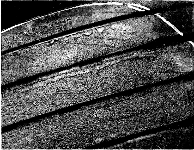
Figure 3.- Reverted-rubber skid patch obtained with four-engine jet transport on wet runway.
