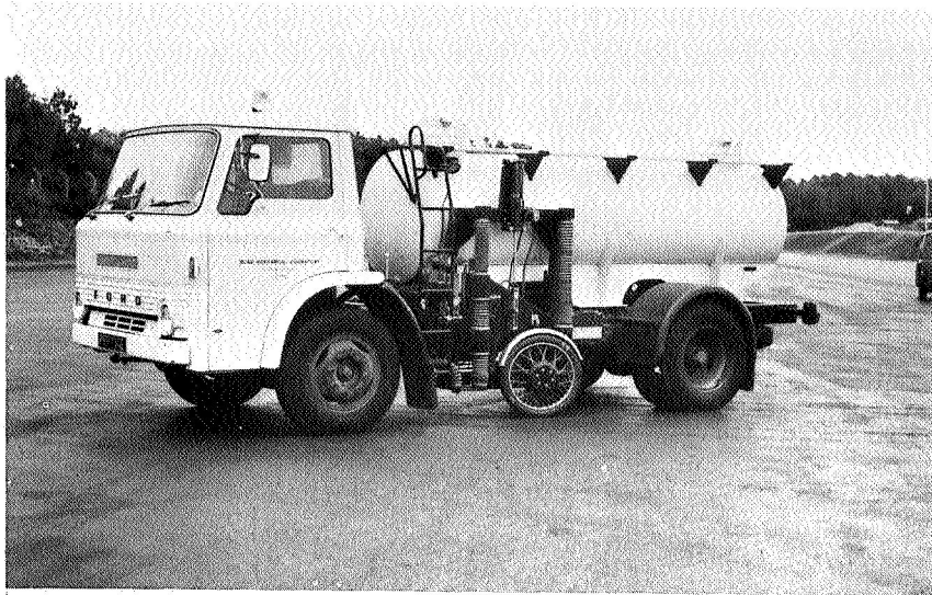
Figure 1.- Skid test vehicle to be used in monitoring the skidding resistance of roads in Great Britain.
