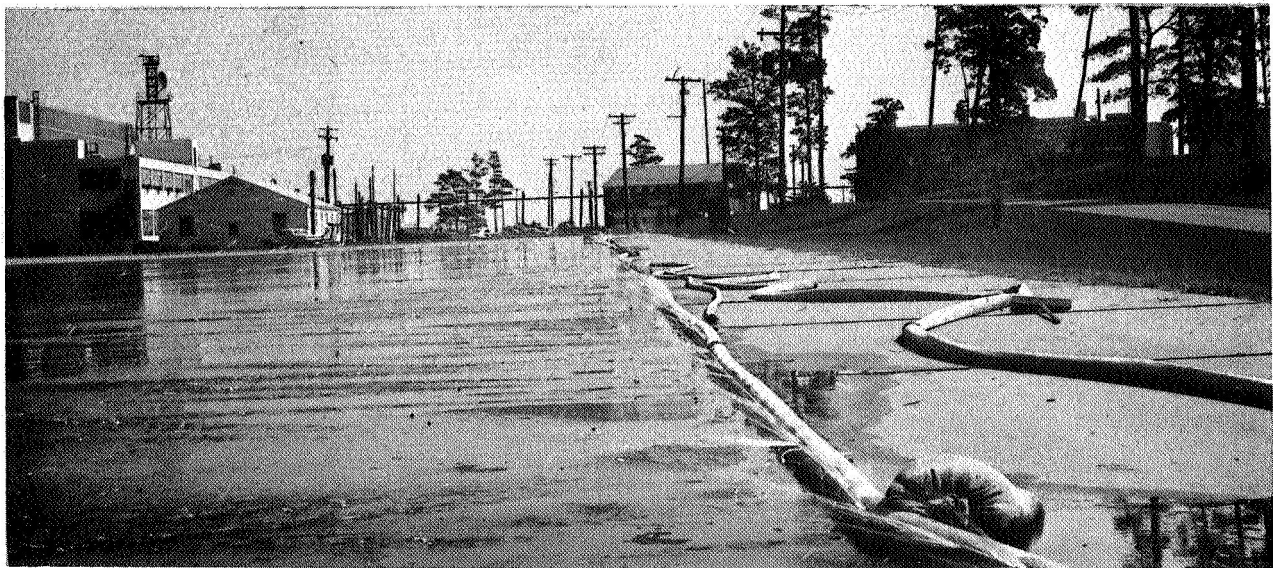
(b) Pierced-canvas-fire-hose sprinkler system used to wet or flood site III skid pad.
