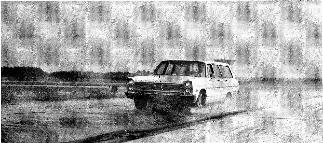
(a) NASA diagonal braking car undergoing test on surface E of site II under a flooded pavement condition provided by plastic-pipe sprinkler system.
