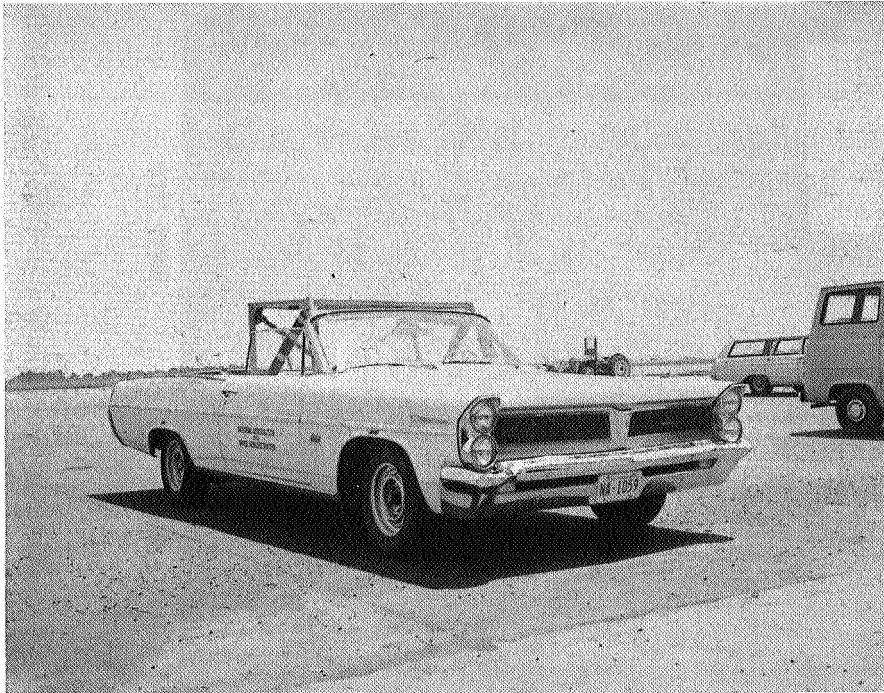
Figure 9.- Stripped convertible with protective cage used by NASA in vehicle spin-out tests on site III skid pad.
