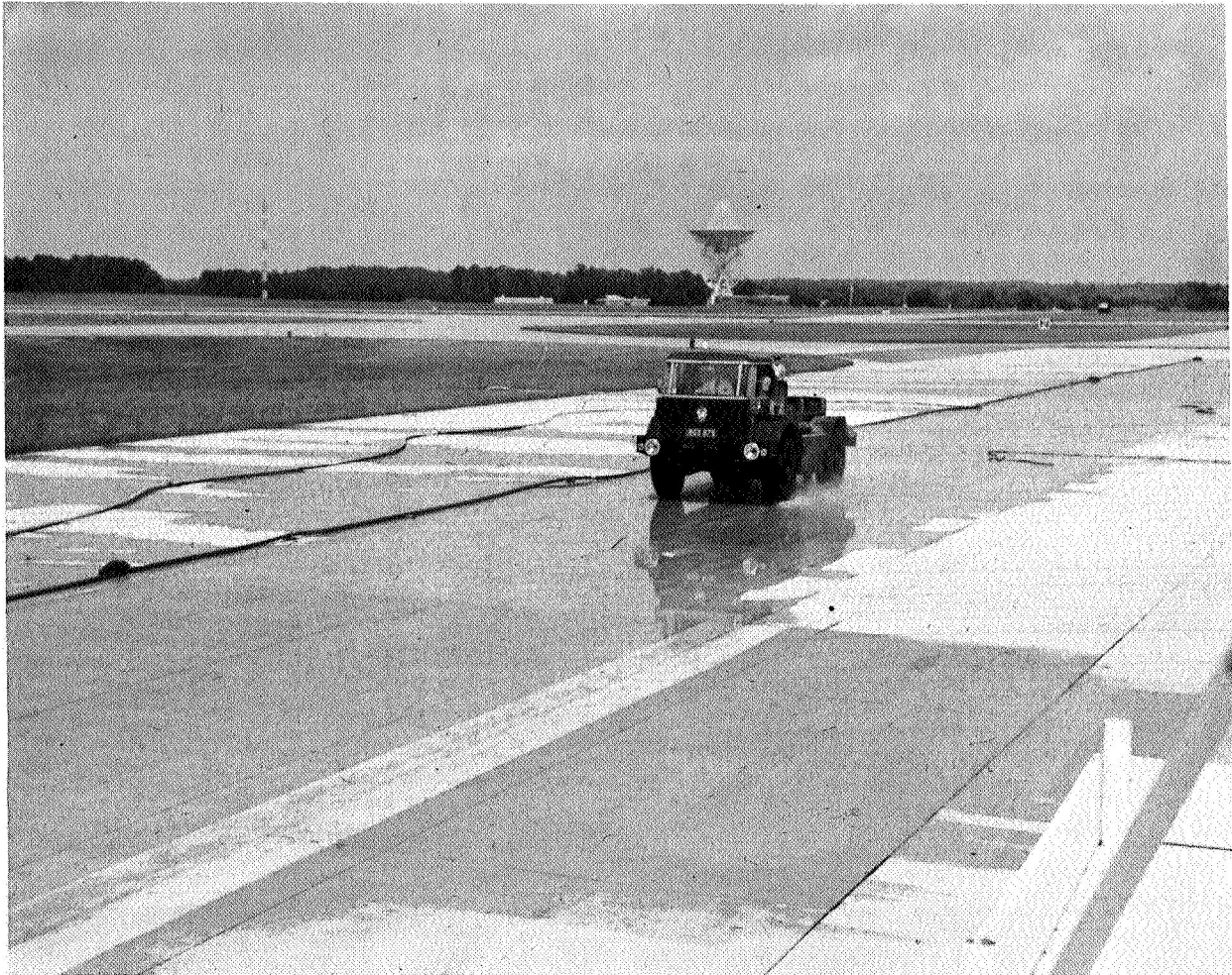
Figure 6.- The British "Juggernaut" test vehicle undergoing a braking test on surface A of site I under a wet and puddled pavement condition.
