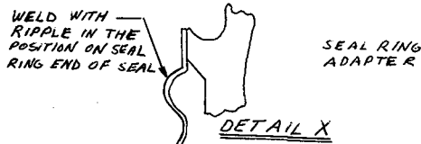
SECTION A-A BELLWS ASS'Y 700405-5 CDJ-83
