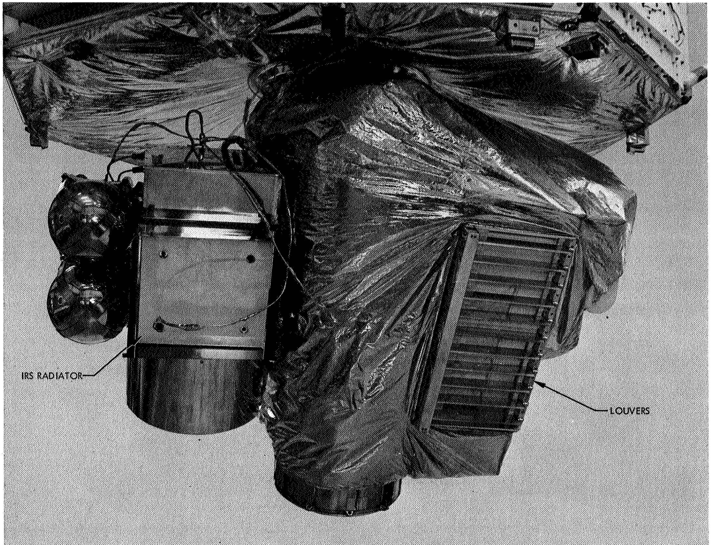
Fig. 4. Platform blanket installed in flight configuration
