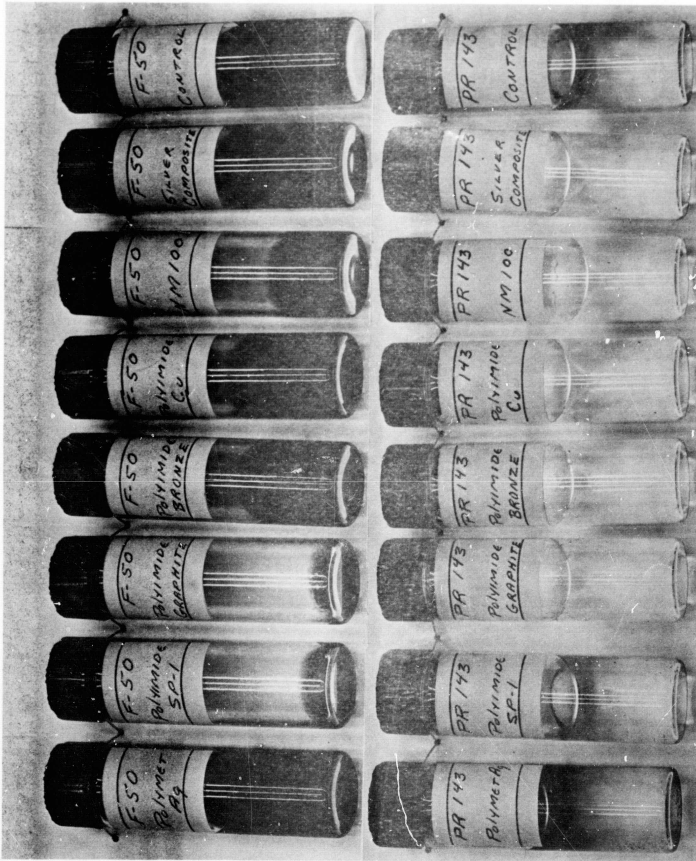
Figure 2-8. F-50 Silicone and PR-143-AB Fluids After Testing at 600°F
