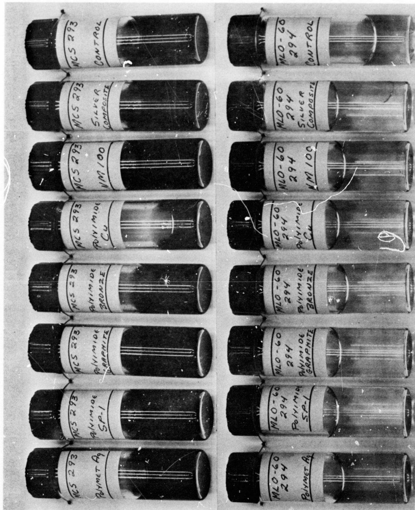
Figure 2-7. MCS-293 and MLO-60-294 Fluids After Testing at 600°F
