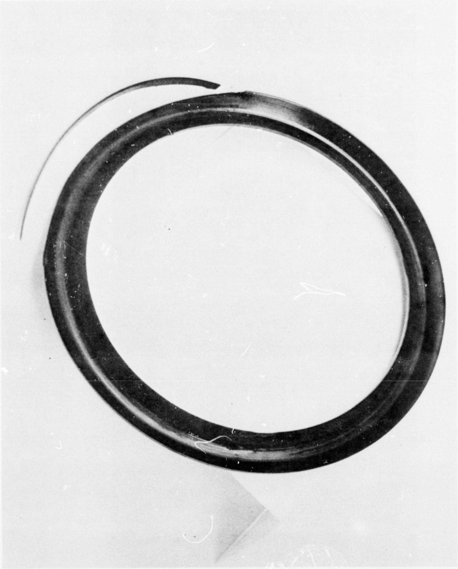
Figure 6-19. Three-Inch Polyimide V-Seal, B-End (Circumferential Cracks)
