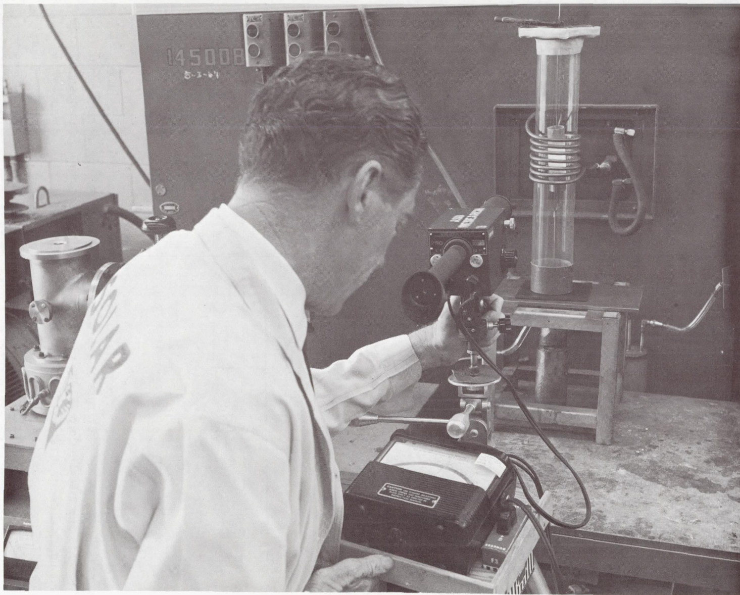
FIGURE 6. APPARATUS FOR BRAZE SEPARATION (REMELT) TEST AND 1750°F TENSILE TESTS OF SHEAR SPECIMENS
