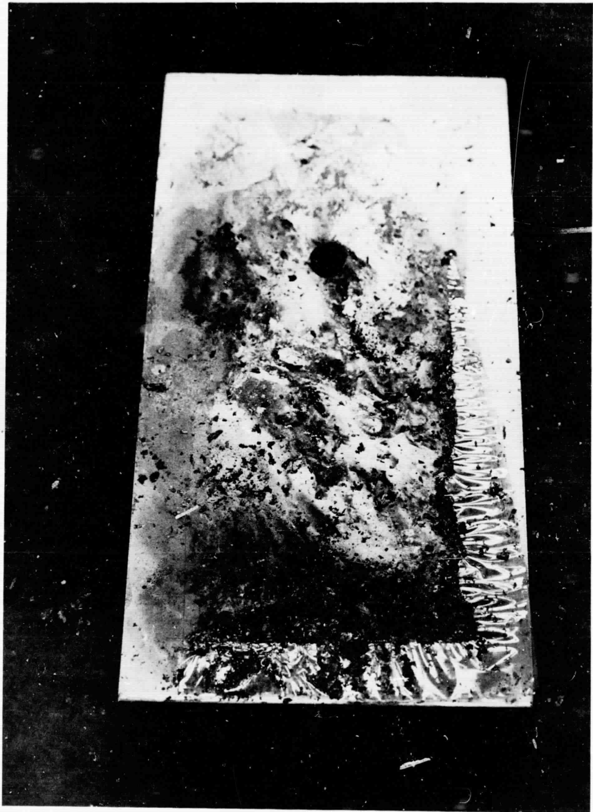
FIGURE 7. SPECIMEN 18 AFTER LOX BALLISTIC IMPACT TESTING
