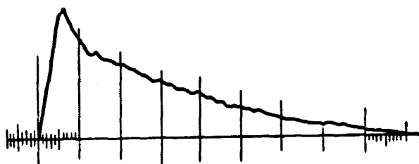
Fig.7. Signal (nT). One division corresponds to 1 \mu second, and nT = 8 \cdot 10^{14} ev \cdot cm ^{-3}
