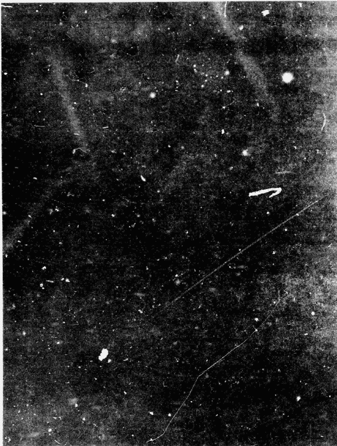
Figure 2 ELECTRONMICROGRAPH OF FLUON GP-1 FILM WITH 43.0% CRYSTALLINITY AT 8,000X; \text{WO}_3 SHADOWED, \text{SiO}_2 REPLICA
