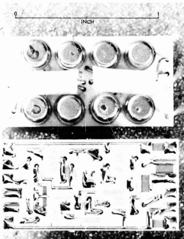
Fig. 25. Thin-film amplifier module, showing individual filter capacitors
