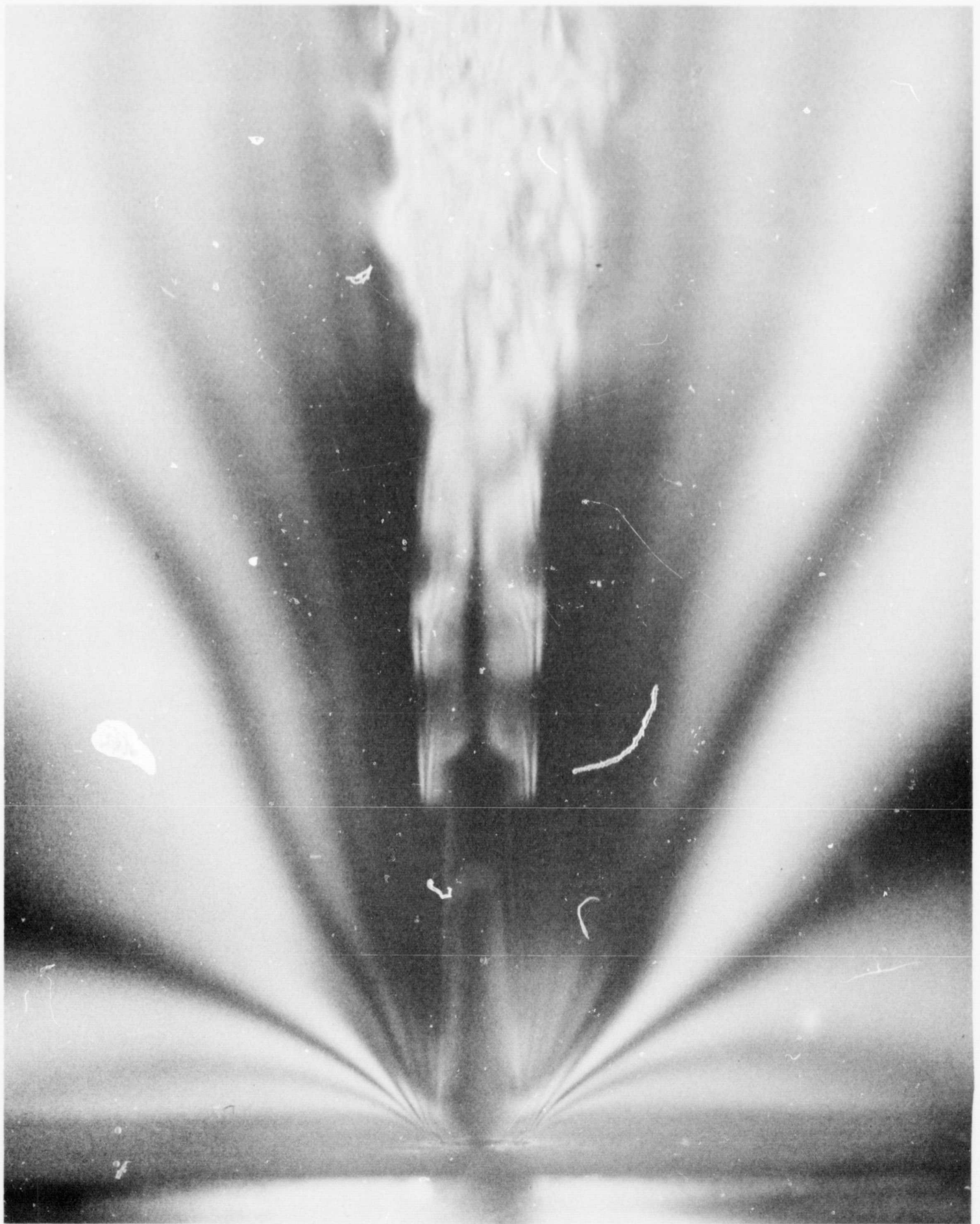
Figure 36. Visualization of a Submerged Liquid Jet Using Flow Birefringence
