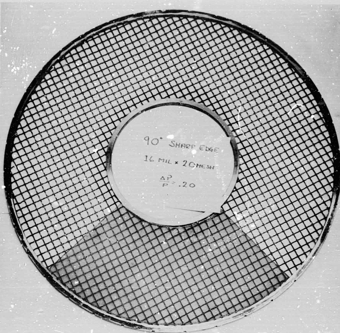
Figure 4(b) - Photograph of heavy 90° circumferential inlet distortion screen mounted on support screen
