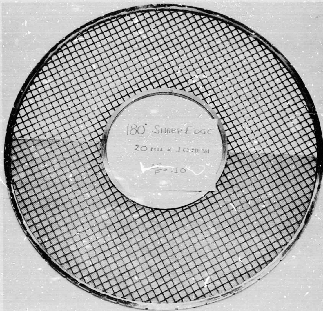
Figure 4 (d). - Photograph of light 180° circumferential inlet distortion screen mounted on support screen.
