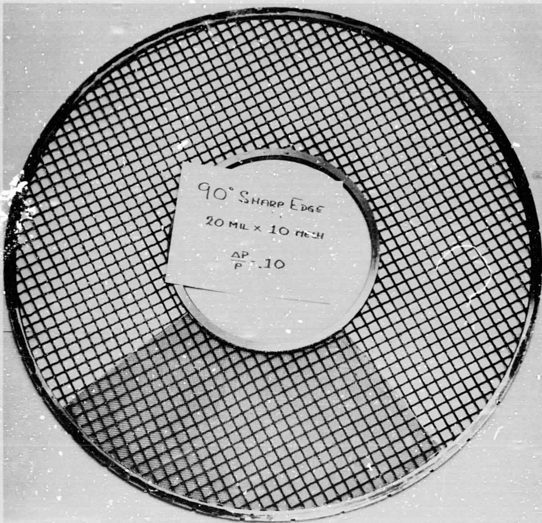
Figure 4 (c). - Photograph of light 90° circumferential inlet distortion screen mounted on support screen.
