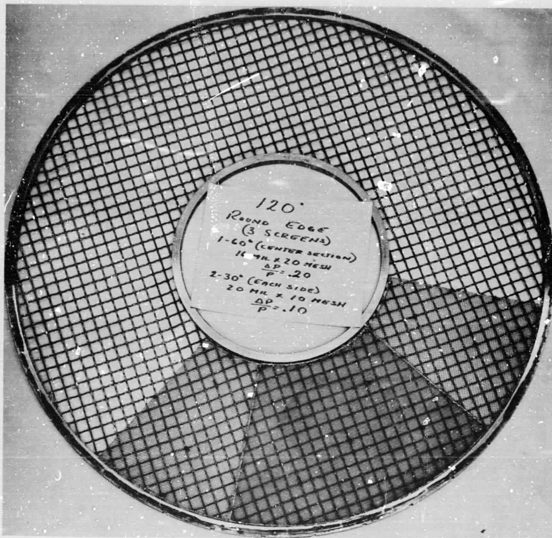
Figure 4 (e). - Photograph of rounded 120° circumferential inlet distortion screen mounted on support screen.
