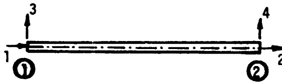
Fig. 2.2 Planar Truss Element
