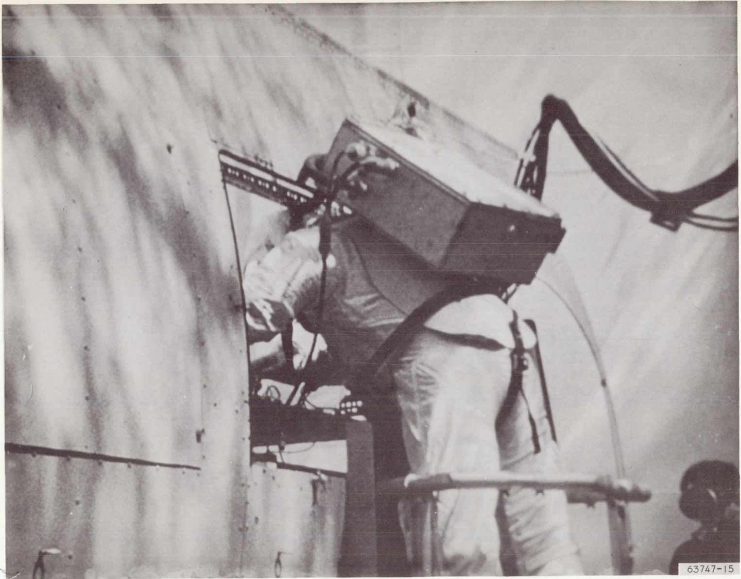
Figure 4-137. Subject Wedging Head and Backpack Against Upper Edge of Access Opening to Maintain Work Position
