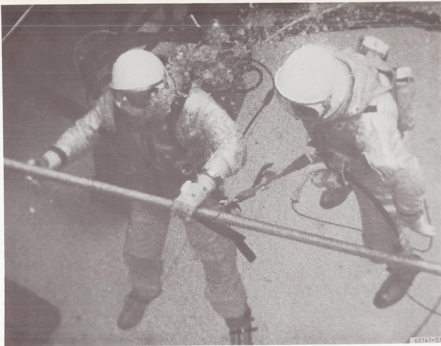
Figure 4-96. Subject Manipulating Dummy Attached to Rail with Strap Tether
