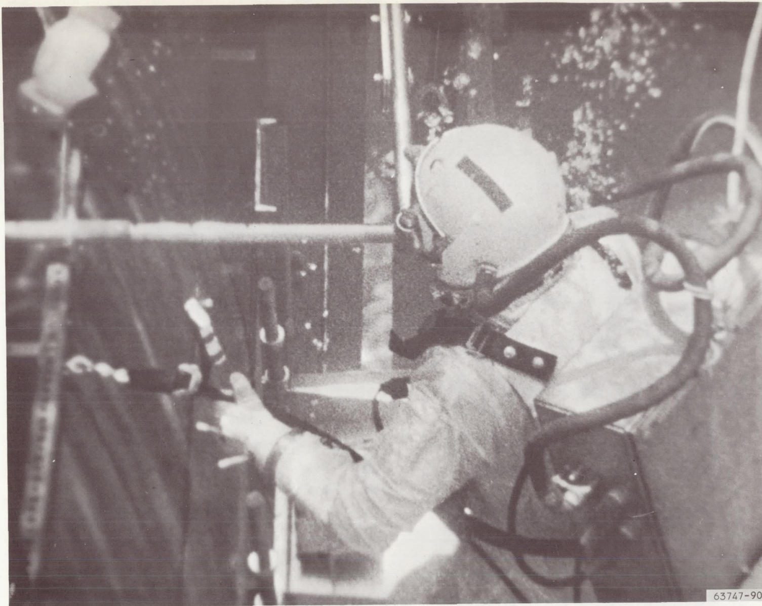
Figure 4-17. Subject Placing Top Support for Panel Holding Jig; Note Strap Tether to Mockup Surface
