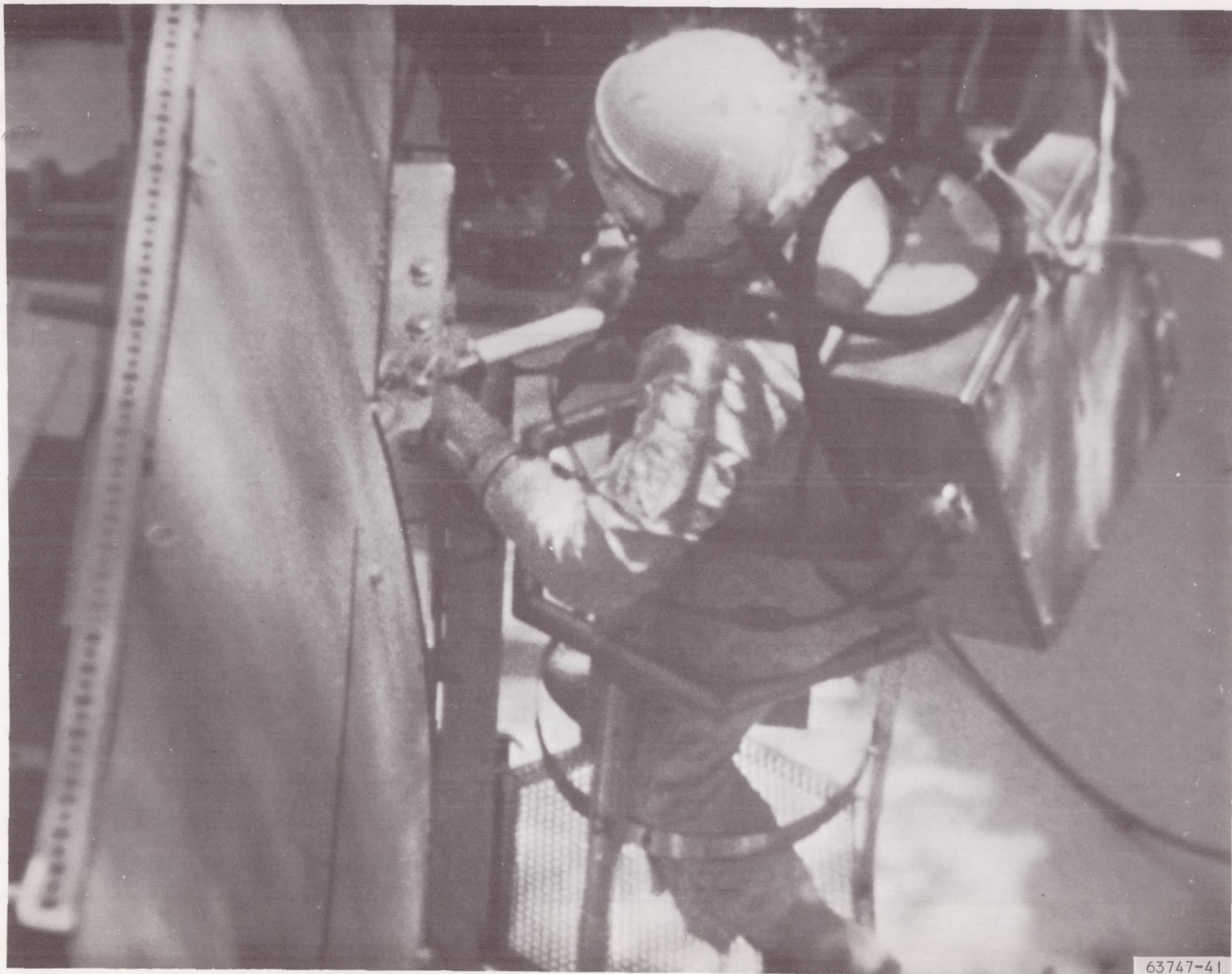
Figure 4-130. Subject Falling Backwards From Wrench Slipping Off the Bolt Head; Cage Restraint Allows Quick Recovery
