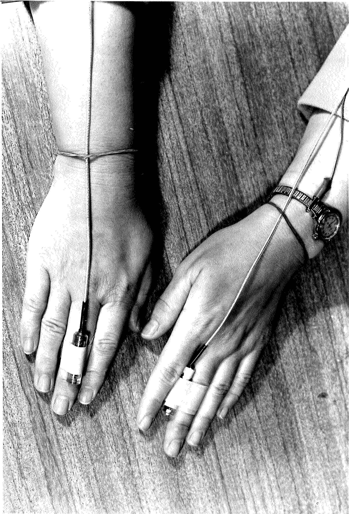
Fig. 2 - Muscle Accelerometers Used to Measure Arm and Hand Motions
