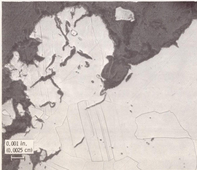
495-Minute exposure at 800° F (427° C).
