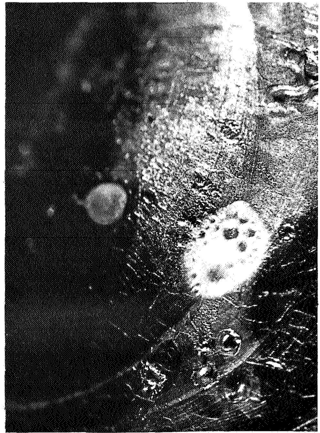
Figure 13. Location of Leak in Weld Nugget of 0.375-Inch Diameter T-111 Tube Removed from Boiler. The Bubbles were Produced by Air Pressurization of Tube with a Soap Film Coating on OD. (C68081422, C68081423, C680814250 Mag.: 10X
