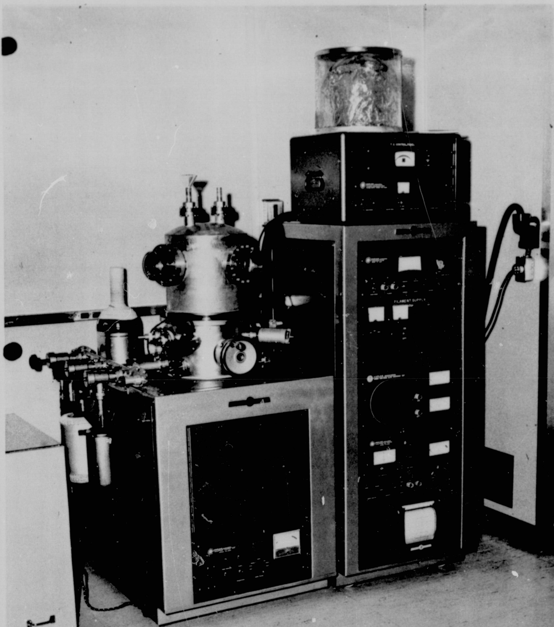
ULTRAHIGH VACUUM UNIT (VARIAN ION PUMP SYSTEM) WITH CRYOGENIC (LIQUID HELIUM) ATTACHMENT IN CLEAN ROOM PREPARATION LABORATORY, RESEARCH INSTITUTES, UNIVERSITY OF CHICAGO, COMMITTEE ON BIOPHYSICS.
