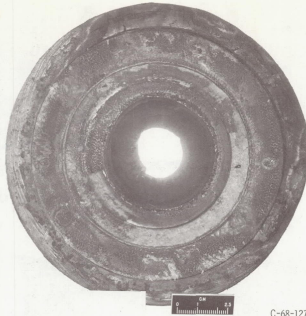
Figure 21. - Graphite-phenolic (FM5064, 60° centerline) after 300-second firing time. Chamber pressure, 100 psia (689 kN/m 2 ); injector 6.
