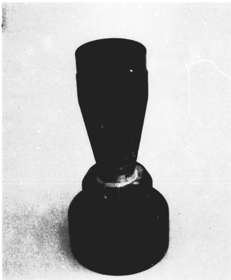
Figure I-9. Side View of Orifice Plate Assembly Showing Exhaust Tube at Top.
