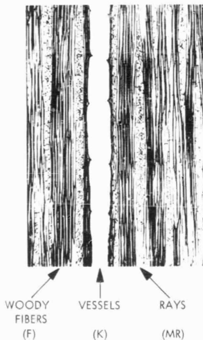
Fig. 3. Photomicrograph of balsa cell structure in a plane parallel to tree axis enlarged 25 times (Photo courtesy of N.Y.S. College of Forestry)
