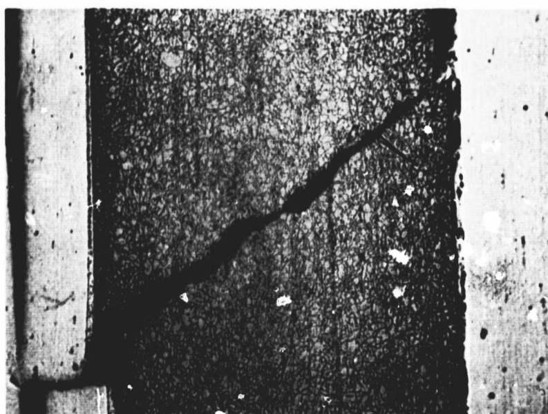
FIGURE 26. FAILURE IN WALL OF DUCT 38, COINCIDENT WITH FATIGUE CRACKS IN STAINLESS STEEL DAMPING SLEEVE
