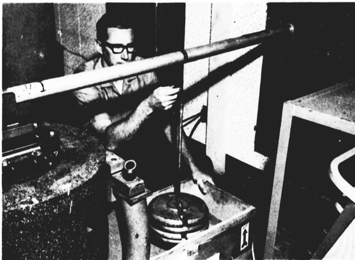
FIGURE 38. METHOD OF RELEASING DEAD WEIGHT LOAD FOR RECORDING OF VIBRATION DECAY
