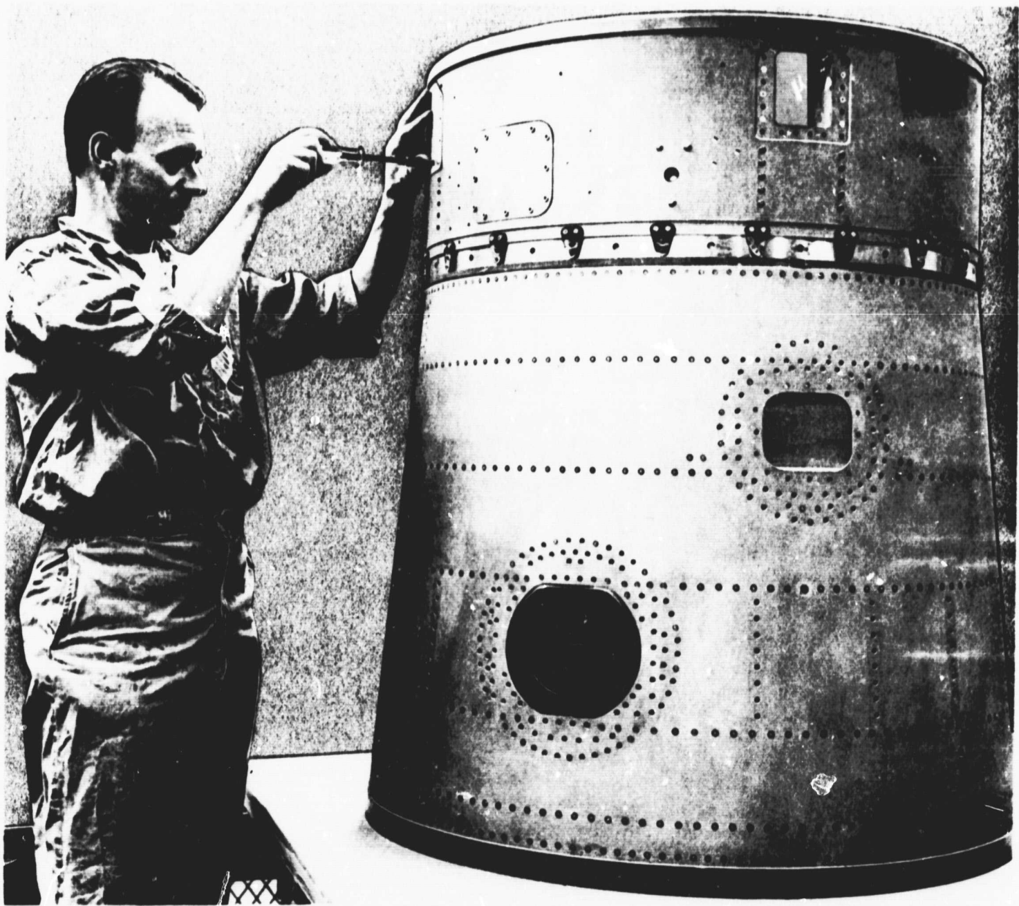
Figure 2-15. Two Beryllium Assemblies for Minuteman: the Spacer (Top) and the Guidance Control Compartment (Bottom) (19)
