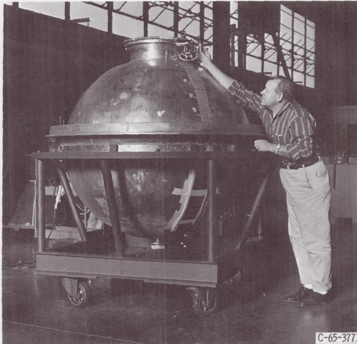
Figure 3. - 1.52-Meter- (5-ft-) diameter spherical test tank. Tank wall thickness, 0.762 centimeter (0.30 in.).
