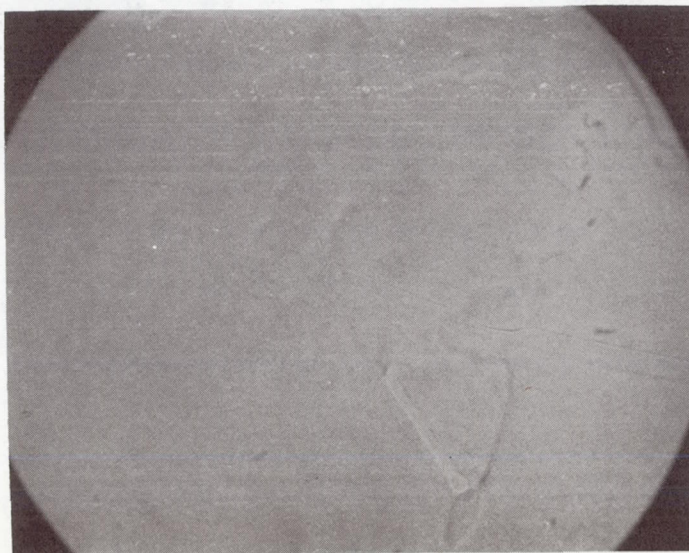
FIGURE 4g. TYPICAL AREA OF EMITTER 1 AFTER HEAT TREATMENT – DIAMETER = 0.19 mm
