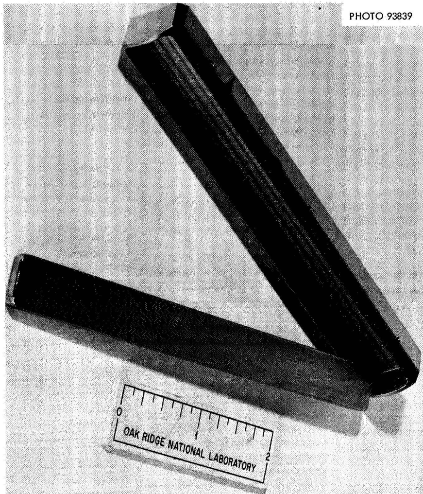
Fig. 6. Flat Plate ^{153}\text{Gd} Source and Shield.
