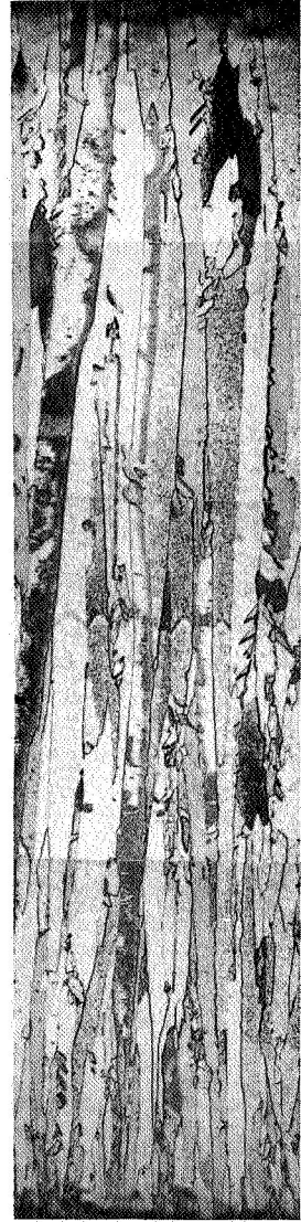
Figure V-11. Cross Section After 20 Minutes at 1900°C, Repolished and Etched. WF5.
