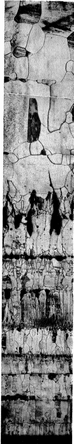
Figure V-34. Cross section of sample WC6B' after 1 hour at 2000 °C.
