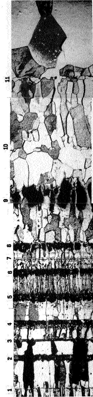
Figure V-24. Cross Section After 1 Hour at 2100°C, Repolished and Etched. WC3B'.
