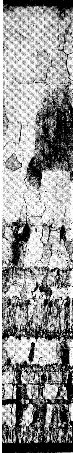
Figure V-32. Cross section of sample WC1A as received. The scale for this figure applies to all other cross sections of this type.
