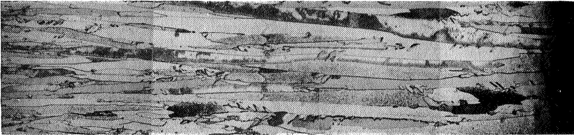
Figure V-14. Cross section of sample WF4B' after 6 hours at 1800°C.
