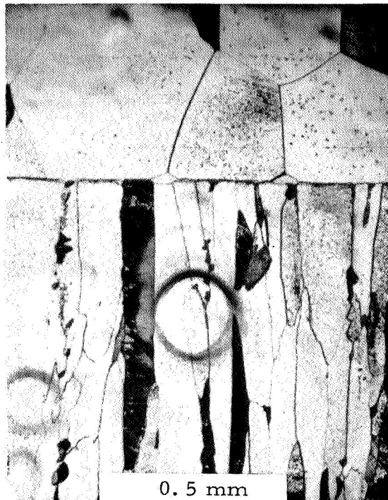
Figure IV-2. Cross-Section of Emitter Showing Columnar Deposit of Tungsten from the Chloride Which Provides Emitting Surface.
