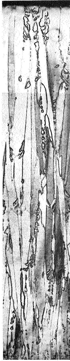
Figure V-11. Cross Section After 20 Minutes at 1900°C, Repolished and Etched. WF5.
