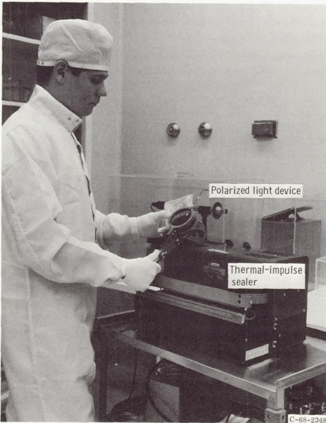
FIGURE 20.—Inspection of seal of clean room packaged part. Typical thermal-impulse sealer is shown.
