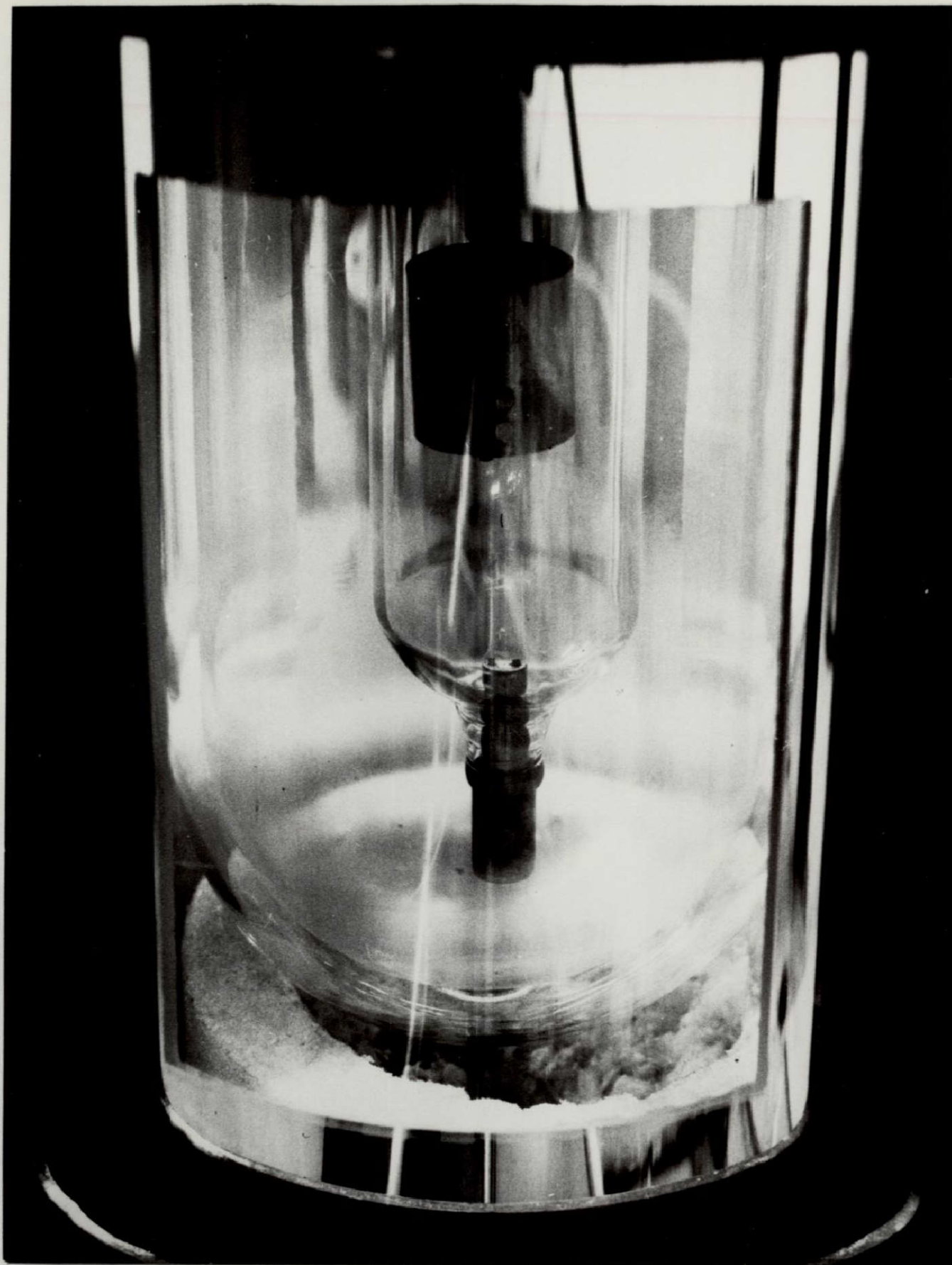
SPECIALLY DESIGNED CRYOSTAT AND ACCESSORIES FOR EVAPORATION OF THIN FILMS IN ULTRAHIGH VACUUM AT LIQUID HELIUM TEMPERATURES
