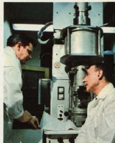
The author created and developed the ultralow temperature electron microscope. Promised improvement can be seen in the photomicrograph, below, which shows the lattice structure of the enzyme, catalase.
