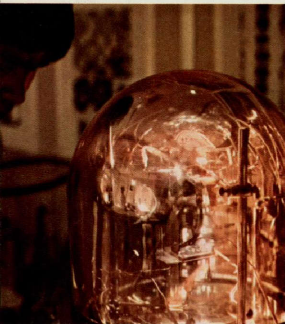
Thin layer of metal is deposited on specimens in ultrahigh vacuum, left . Photographic laboratory, above , includes shadowgraph on which projected image from the microscope can be studied in detail.
