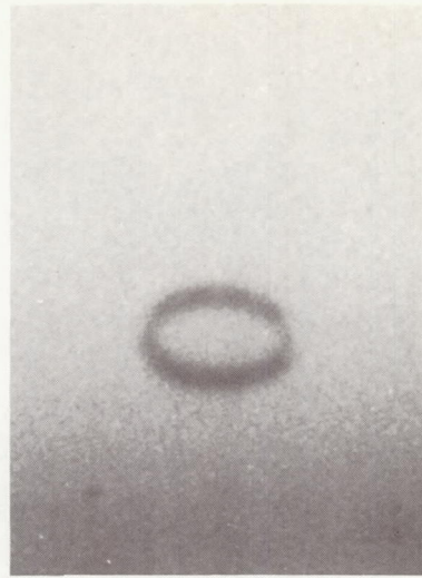
(b) Test liquid, methanol; acceleration, 18.2 centimeters per second squared; equivalent radius, 0.26 centimeter; distortion parameter, 1.50; terminal velocity, 8.9 centimeters per second.
