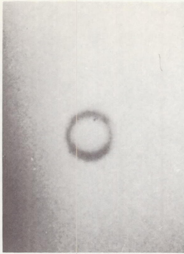
(a) Test liquid, 1-butanol; acceleration, 12.0 centimeter per second squared; equivalent radius, 0.21 centimeter; distortion parameter, 0.94; terminal velocity, 3.7 centimeters per second.
