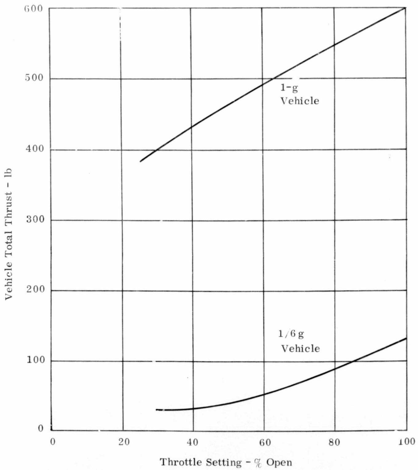
Figure 5. Vehicle Thrust
