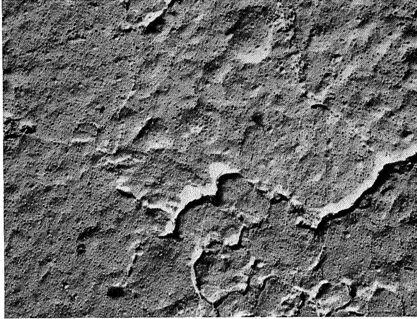
Figure 24: ELECTRON MICROGRAPH (8000X) OF SOLAR CELL SURFACE
